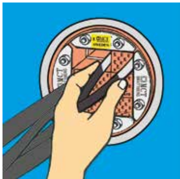
5 Tweezers can be used, if required, to aid installation of last row of blocks.
